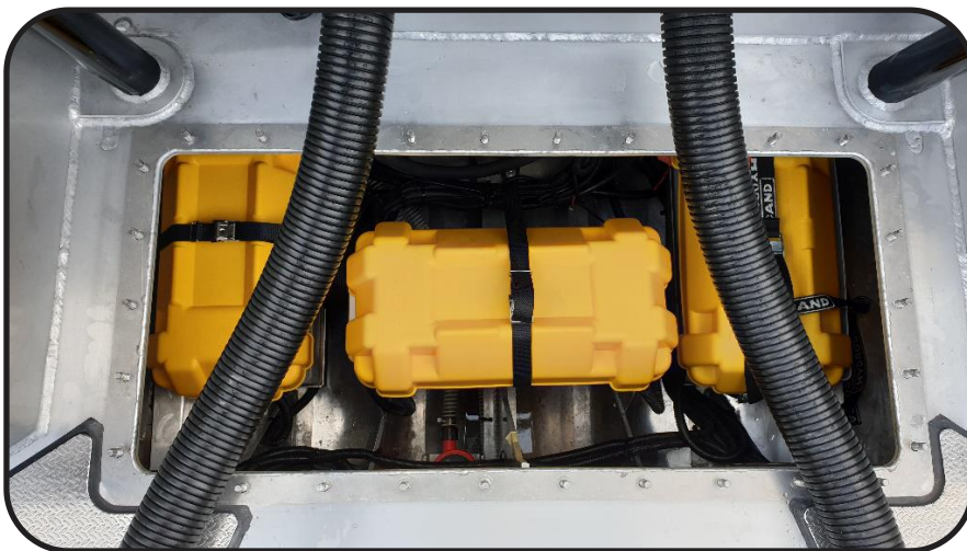
Battery compartment with maximum 3 batteries, shown with hatch open.
