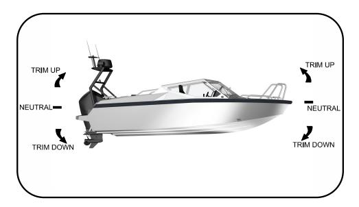
The engine trim is used to adjust the bow up or down (the so-called pitch) while the boat is under speed. A well-adjusted engine trim will maximize safety and comfort, and will minimize fuel consumption.
